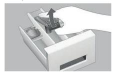
Release the blue insert by lightly lifting it up and take it out of the detergent drawer.
