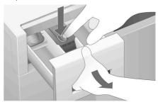
Press down the blue tab in the compartment and pull the drawer all the way out.
