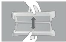
Pull out the outer coarse filter
